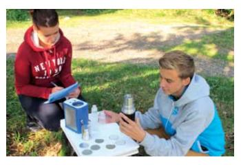
The membrane filtration method involves filtering a water sample using membrane filters of a standard pore size, placing each filter in a Petri-dish on a pad saturated with nutrient medium and incubating at a specific temperature. After incubation, bacterial colonies that have grown on the membrane are counted.
