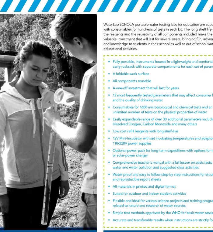
High turbidity points to the presence of microorganisms and other potential contaminants that could be of health concern. A collected water sample is gradually poured into the turbidity tube until the cross at the bottom of the tube just disappears.
